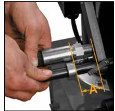
Hold the fitting against the Coupling Stop Arm withdraw the Coupling Stop Rod such that the Guide is aligned with the desired crimp position. Lock the Coupling Stop Clamp.
